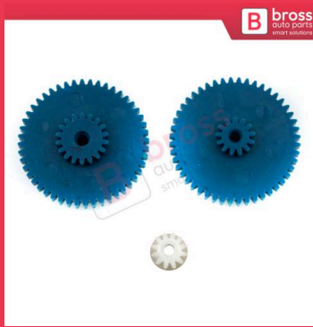
BGE36 Speedometer Euro KM Odometer Gears for Mercedes W124 E500 W126 W107 560SL
