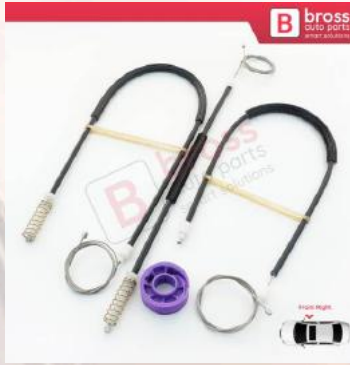
BWR5079 Power Window Regulator Repair Set Front Right Door for Seat Toledo MK3 5P2 2004-2009 Altea 5P1 XL 5P5 5P8 5P0837462
