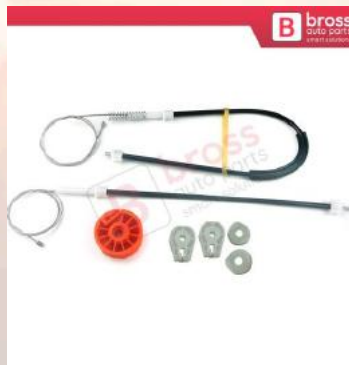
BWR566 Power Window Regulator Repair Set Rear Right for Renault Megane MK2 EM0/1 2002-2009 CC Cabriolet Convertible 8201010932
