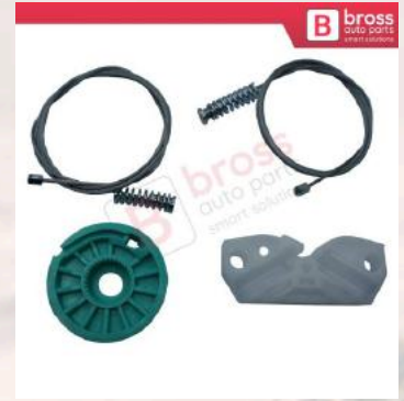
BWR1119 Window Regulator Kit Rear Quarter Window Left Door for Mercedes CLK C209/A209 2002-2009
