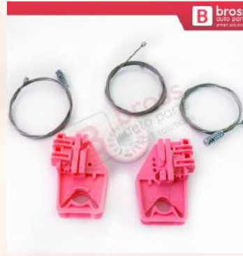
BWR567 Power Window Regulator Repair Set Front Left for Skoda Octavia MK2 A5 1Z3 1Z5 2004-2013 4/5-Door 1Z1837461
