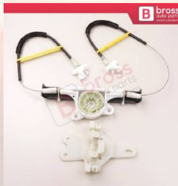
BWR5142 Window Regulator Repair Kit Rear Left Door for Nissan Terrano MK2 1993 2005 4/5 Doors
