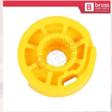
BWR843 Window Regulator Wheel Front Left Door for Audi A3 A4 A6
