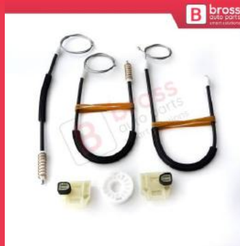
BWR5389 Window Regulator Repair Set Front Door for Seat Leon MK1 1M1 1999-2006 Seat Toledo MK2 1M2 1998-2004 4/5 Door 1M0837461A 1M0837462A
