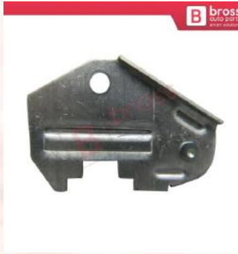
BWR5008 Window Regulator Clips Metal Connection Sheet Left Doors for Vauxhall Opel Vectra Saab 9-3
