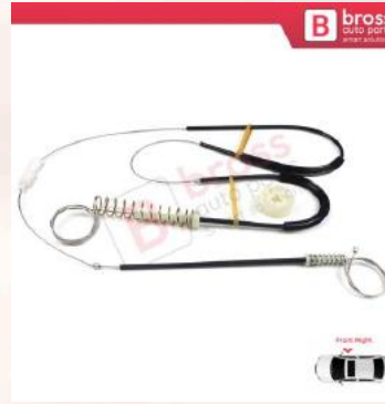
BWR5163 Window Regulator Repair Set Front Right Door 8N0837462 for Audi TT MK1
