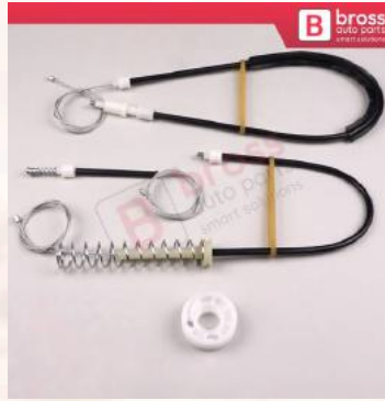
BWR1032 Window Regulator Repair Kit Rear Left Door for VW Phaeton Lounge 2005-On
