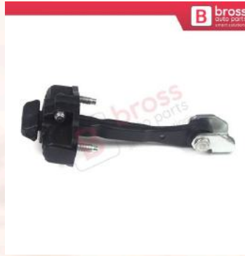
BDP830 Front Door Hinge Stop Check Strap Limiter 50509843 for Alfa Romeo Giulietta 940 2010-2020
