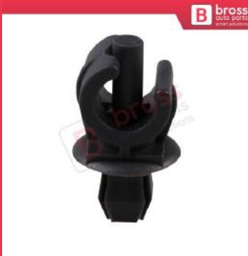
BCF1829 10 Pieces Retainer for VW Stem Diameter 4.3 mm Fits Into 7.5 mm Hole Overall Height 26mm
